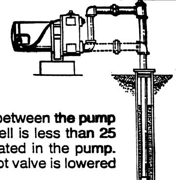
Where the vertical distance between the pump and the water level in the well is less than 25 feet, the injector is incorporated in the pump. Only a suction pipe with a foot valve is lowered into the well.
